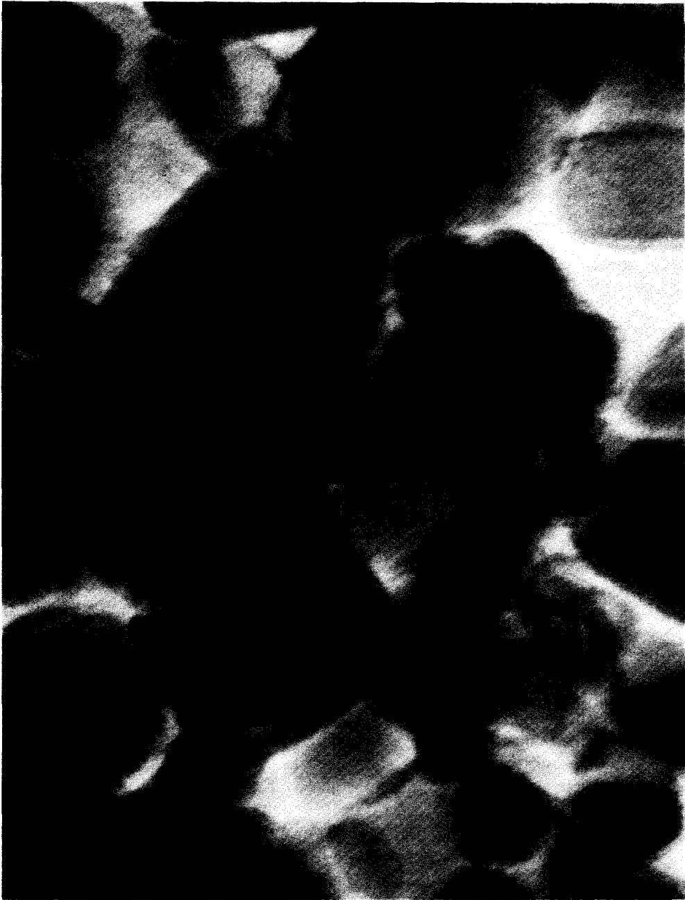
FIG. 4. Transmission electron micrograph of blank \text{TiO}_2 following hydrogen reduction at 770 K.
